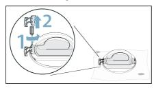
**5.** Remove the screws from the eyelet and remove the eyelet.
