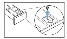
Turn the condensation container 180° onto its underside and insert the stopper.
