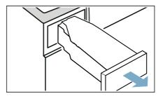
2. Remove the filter and clean it under running water or in the dishwasher.
