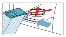
Note: If you pour more than 180 ml drinking water into the appliance and Refresher-container is empty, please re-fill. does not go out on the display, this means that the drinking water has been poured into the wrong filling hole or the appliance is not fully level. Pour the drinking water into the filling hole on the front or make the appliance level.
