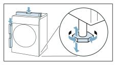
If necessary, turn the appliance feet to make sure it is level.You can now connect the appliance.
