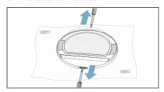
9. Remove the side parts of the door.
