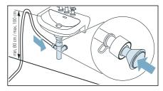
The connection point must be secured using a hose clamp (12-22 mm clamping range, available from specialist retailers).
