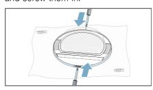
**12.** Rotate the door ring by 180° and insert the door properly.
