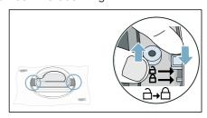
14. Screw the hinge onto the door.
