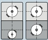
The front and rear hotplates each have two inductors and can be used independently of each other. Select the required heat setting for each of the hotplates. Use only one item of cookware on each hotplate.
