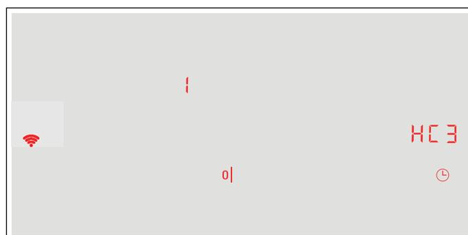
4. Set the **0** value on the control panel. This deactivates Wi-Fi; the Wi-Fi symbol will go out on the control panel.
