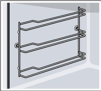
1. Lift the rail slightly at the front **a** and detach it **b** (figure **1**).
