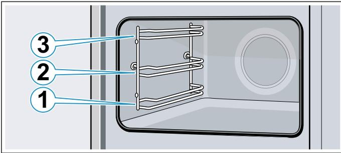
Always insert the accessory between the two guide rods for a shelf position.
