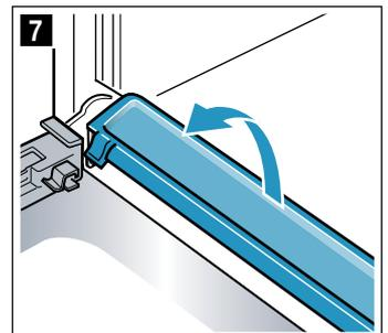
Clean the panels with glass cleaner and a soft cloth. Wipe the condensate trough with a cloth and some hot soapy water.
