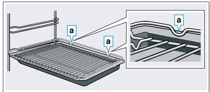
Small steam containers may only be placed in the cooking compartment with the wire rack.
