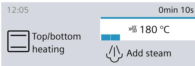
The »»» symbol appears on the left next to the temperature. The temperature indicator starts to fill in.
