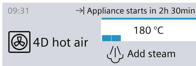
The oven is in standby. The →| symbol and the time when the operation will be finished appear in the status bar. The operation starts at the appropriate time. You can see the cooking time counting down in the status bar.
