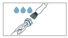
4. Connect the hose and check for leaks.
