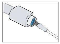
Connect the water inlet hose and check for leaks.
