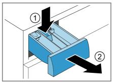
Press out the insert upwards from below.
