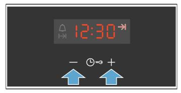
The appliance will apply the settings after a few seconds. The end time will be shown on the display. Once the appliance starts, the time will begin counting down.
