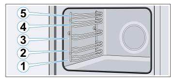
Always insert the accessory between the two guide bars for a shelf position.
