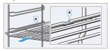
When inserting baking trays, make sure that the recess **a** is at the rear and is facing downwards. The sloping edge of the accessory **b** must be facing towards the appliance door.
