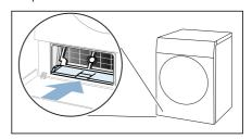
**11.** Slide the heat exchanger cover in by its grip.
