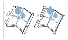
Dry the two parts of the fluff filter, snap them shut and reinsert the filter.
