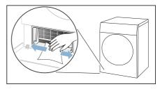
**Note:** Take care not to damage the heat exchanger, as it is exposed.
