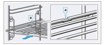
When inserting baking trays, ensure that the catch tappet **a** is at the rear and is facing downwards. The sloping edge of the accessory **b** must be facing forwards towards the appliance door.
