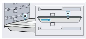
Do not push the steam container out via the recess
