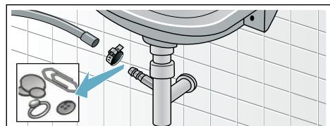
4. Re-attach the drain hose and secure the connection point using the hose clamp.
