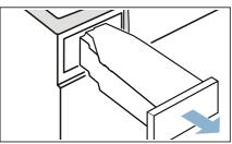
2. Push the condensation container back into the appliance until you feel it lock into place.
