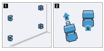
Use the hook to attach the rear holder into the upper hole a and push it into the lower hole b (fig. ☑).
