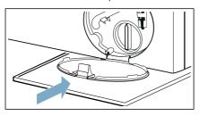
**Note:** To prevent unused detergent from flowing straight into the drain during the next wash: Pour 1 litre of water into dispenser **II** and start the **Empty** programme.
