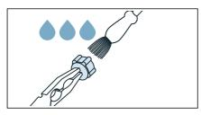
Connect the hose and check for leaks.
