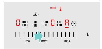
The function has now been activated. The 1 temperature symbol will remain lit until the frying temperature has been reached. An audible signal sounds and the temperature symbol goes out.
