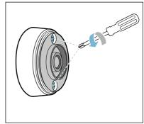
2. Open the closure of the temperature sensor. Remove the battery from the lower section of the housing and insert a new battery (pay attention to the correct orientation of the battery poles).
