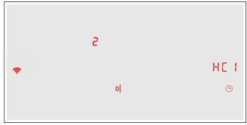
Use the "Home Connect" SSID and the "Home Connect" key to log your mobile device into the hob network.
