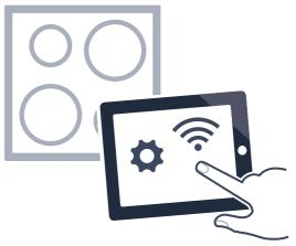
If the range symbol no longer flashes in the control panel but, instead, lights up constantly, the hob is connected to the home network.
