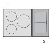
**Note:** In the combi zone, the PowerBoost function can only be activated if the two hotplates are used independently of each other.
