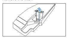
Clean the filter under warm, running water or in the dishwasher. **5.** Push the filter in until you feel it lock into place.
