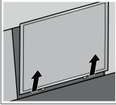
**Note:** Fat may accumulate in the bottom of the filter holder. Hold the filter holder at an angle to prevent fat from dripping out.
