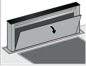
4. Remove the filter from the guide.
