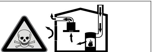
Room air-dependent heat-producing appliances (e.g. gas, oil, wood or coal-operated heaters, continuous flow heaters or water heaters) obtain combustion air from the room in which they are installed and discharge the exhaust gases into the open air through an exhaust gas system (e.g. a chimney).
