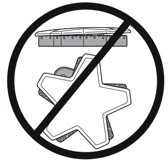
Incorrect burner cap
