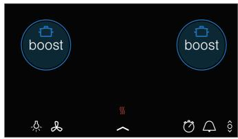
If the powerBoost function is activated and you configure the settings for a different cooking zone on the same side of the cooking surface, the powerBoost function will be deactivated and power level 9.0 selected automatically.
