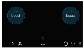
If the panBoost function is activated and you configure the settings for a different cooking zone on the same side of the cooking surface, the panBoost function will be deactivated and power level 9.0 selected automatically.
