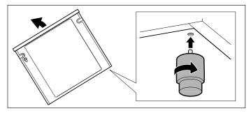
**Note:** If the appliance needs to be moved again, screw the adjustable feet in fully.
