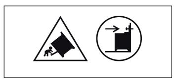
**Warning:** In order to prevent tipping of the appliance, this stabilizing means must be installed. Refer to the instructions for installation.
