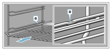
When inserting baking trays, ensure that lug  $\mathbf{a}$  is at the rear and is facing downwards. The sloping edge of the accessory  $\mathbf{b}$  must be facing towards the appliance door.
