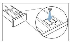
10. Pull the filter out of its snap-in lock.
