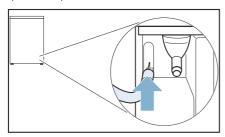
5. Take the drain hose from the accessories and attach it to the free socket, pushing it up to the stop.
