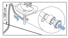
The connection point must be secured using a hose clamp (clamping range 12-22 mm).
