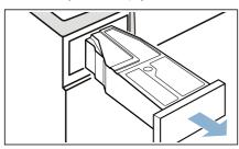
Push the condensation container back into the appliance until you feel it lock into place.
