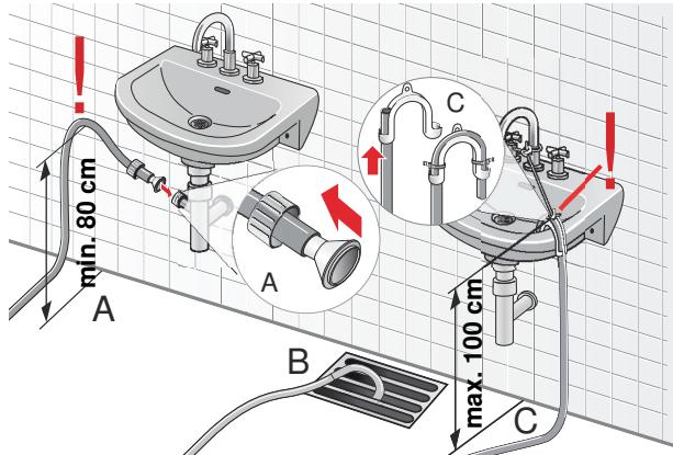
Depending on how you connect the hose (A, B or C), fit the drain hose with the remaining accessories. Check the dimensions.
