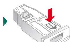
Pull the filter out of its snap-in lock.
