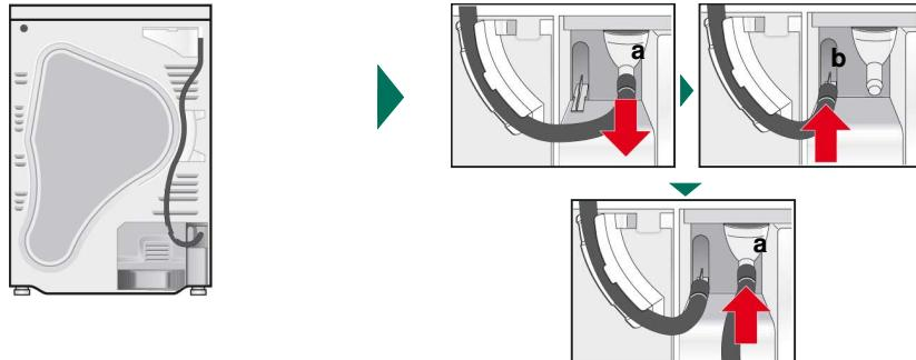
When the dryer is delivered direct from the factory, the hose for discharging the condensation into the condensate container is fastened to the adapter.
