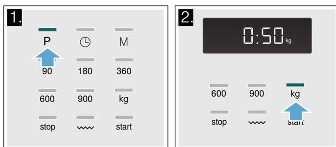
3. Use the control panel to specify the weight of the dish.
