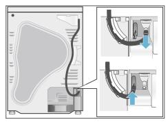
4. Take the drain hose from the accessories and secure it to the free connecting piece.
