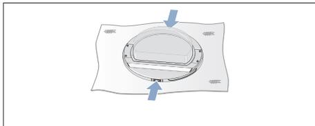
12. Screw the rings tightly back onto the dryer door.
