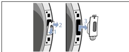
17. Insert the door lock (1.) on the other side of the dryer and screw the cover (2.) back on.
