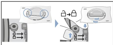
14. Put the door hinge and door handle in place as shown in the picture, and screw them back onto the dryer door.
