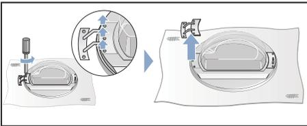
5. Remove the screws from the door handle on the dryer door and remove the door handle.
