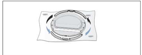
11. Press the rings onto the dryer door.
