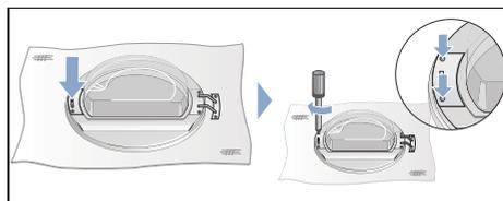
15. Remove the cover from the door lock on the dryer and place it to one side.
