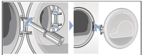
3. Carefully place the dryer door onto a flat surface, and place a hand towel or other such item between the door and the surface to avoid scratching or damaging the door.
