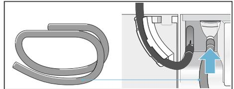
5. Fasten the other end of the drain hose with the remaining accessories, depending on the connection situation (A, B or C).
