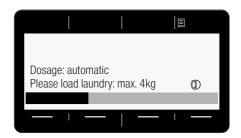
The load bar fills as the laundry is loaded. If the maximum load is exceeded, the bar flashes. Observe the maximum indicated load. Overfilling adversely affects the washing result and encourages creasing.
