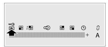
$\boldsymbol{c}$  and  $\boldsymbol{l}$  flash alternately in the left-hand display;  $\boldsymbol{l}$  lights up in the right-hand display.
