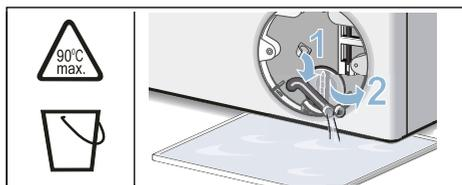
5. Carefully unscrew the pump cover; residual water may leak out. Clean the interior, pump-cover thread and pump housing. The
