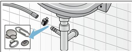
4. Reattach the drainage hose and secure the connection using the hose clamp.
