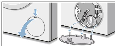
4. Take the drain hose out of the retainer. Remove the sealing cap and pour the water out into a suitable container. Replace the sealing cap and place the drain hose back in the retainer.
