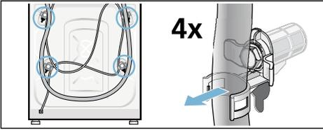
2. Unscrew and remove the bolts from all four transport safety devices. Remove the sleeves. To do this, remove the mains cable from the holders.
