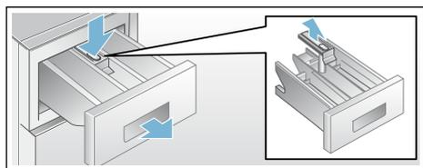
3. Clean the detergent dispenser tray and insert with water and a brush, and dry it. Clean the inside of the housing as well.
