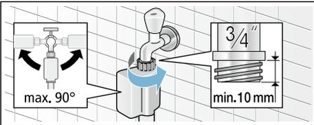
**Note:** Carefully turn on the tap and check that the connection points are not leaking. The screw connection is under water pipe pressure.
