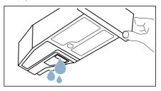
3. Push the condensation container back into the appliance until you feel it lock into place.
