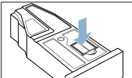
**12.** Skjut in kondensattanken så att den snäpper fast.
