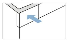
**Note:** The filter in the condensation container filters the condensation water, which is used during the appliance's automatic cleaning cycle. The filter is cleaned by emptying out the condensation water. You should still check the filter regularly for any buildup, and remove this if necessary.
