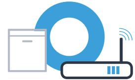
During manual connection, your dishwasher sets up its own Wi-Fi network (access point), which you can log into using your smartphone or tablet.
