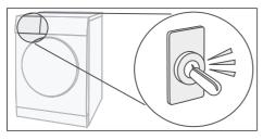
The condensation is pumped into the condensate container using a pump. This generates pumping noises.
