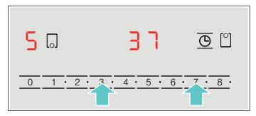
**5.** Touch the  $\bigcirc$  symbol for 4 seconds. The setting is activated.
