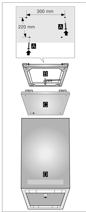
2. Insert the two bolts on the ceiling through the openings provided in the frame A. Move the frame to allow the bolts to be screwed into the keyhole openings B.
