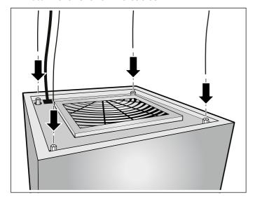
3. Taking care to comply with the safety clearances, slide the appliance up and level it.
