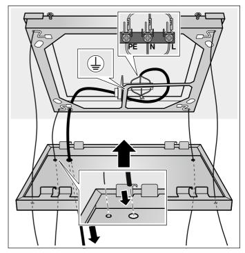
Fit the frame cover onto the four bolts at the edge of the frame.
