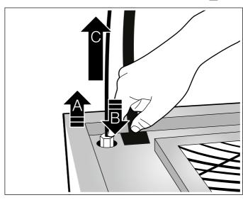
5. After aligning, tighten the cable tensioners so that they are hand-tight. Do not use any tools.
