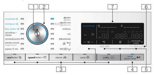
**Note:** All the buttons are sensitive (except for the main switch) and only need to be pressed lightly.
