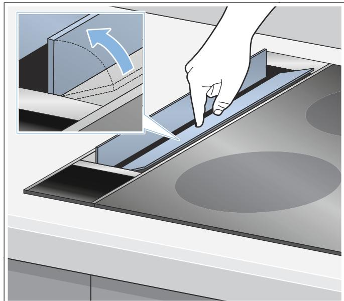
2. Take hold of the metal grease filter with two fingers at its edge and remove it.
