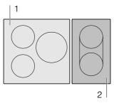
Note: In the combi zone, the PowerBoost function can only be activated if the two hotplates are used independently of each other.
