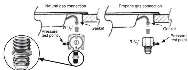
Direction of gas flow is indicated on the rear of the regulator.
