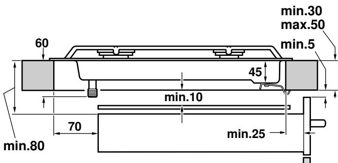
If an oven is positioned below the cooktop the barrier does not need to be fitted, but a space of 35 mm must be maintained between the underside of the cooktop and the top of the oven.
