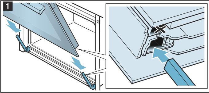
2. Open the appliance door fully. Fold both locking levers closed again (figure 2).
