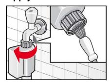
If no water runs into the washer-dryer, or only an insufficient amount, you must first reduce the water pressure in the supply hose:
