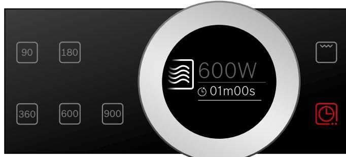
The microwave output and a default cooking time are shown in the display. The field lights up red.
