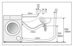
**Note:** If the hose holders are used, the possible hose lengths are reduced!
