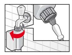
If no water runs into the washer-dryer, or only an insufficient amount, you must first reduce the water pressure in the supply hose:
