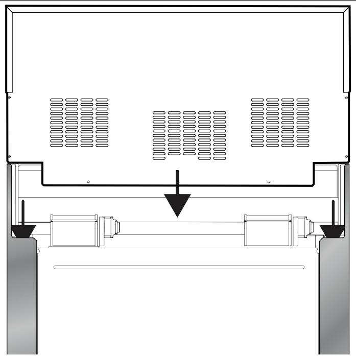
5. Make sure the backguard's front face is outside the flange on the front side of the range.
